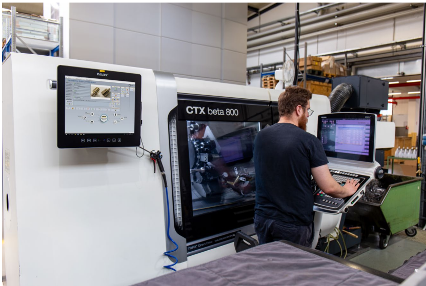
Image 3: The machine park at BERG comprises a total of 18 turning and milling centers as well as grinding machines. Production data is visualized via COSCOM InfoPOINT VM terminals directly at the NC machines.
