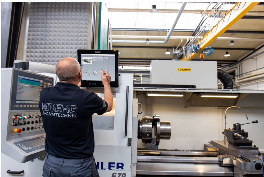
Image 6: On the digital setup sheet displayed at the InfoPOINT terminals, operators can see all the information they need to process the job.
