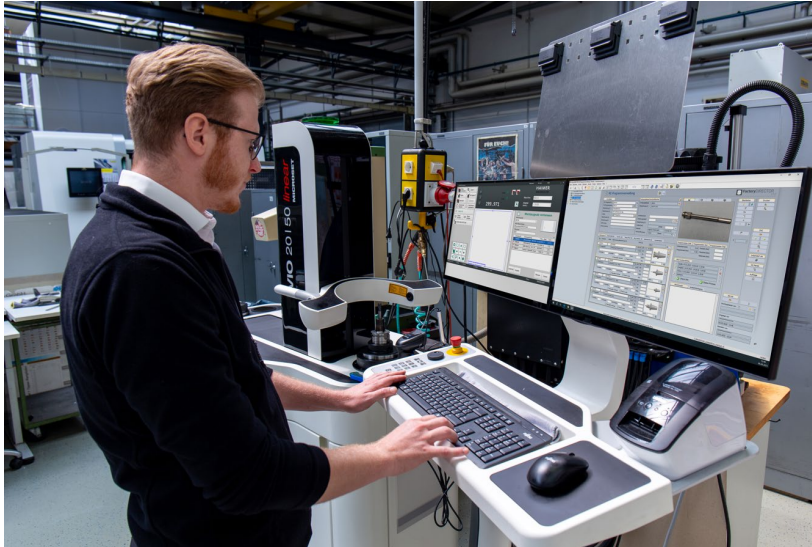
Image 5: The HAIMER tool presetting device is also integrated into the process and exchanges data with the central COSCOM tool management module, ToolDIRECTOR VM, from the setup center.
